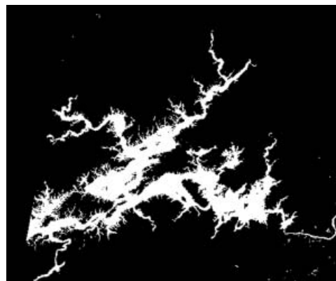
Figure 7. The result of discrimination function. (White indicates that the point is regarded as a lake pixel.)
