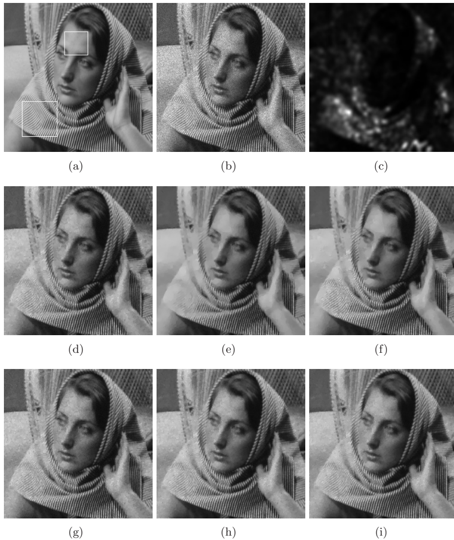
Figure 5. (a) The original “Barbara” image, the marked rectangles are marked for zooming; (b) the noisy image; (c) \lambda(x, y) computed by the spatially varying parameters method; the denoised images: (d) the AA model with \lambda = 1900 ; (e) the AA model with automatic selection of parameter; (f) the spatially varying parameters method; (g) the RLO model; (h) the RISS model with \lambda = 10 ; (i) the HNW model with \lambda = 6 .
