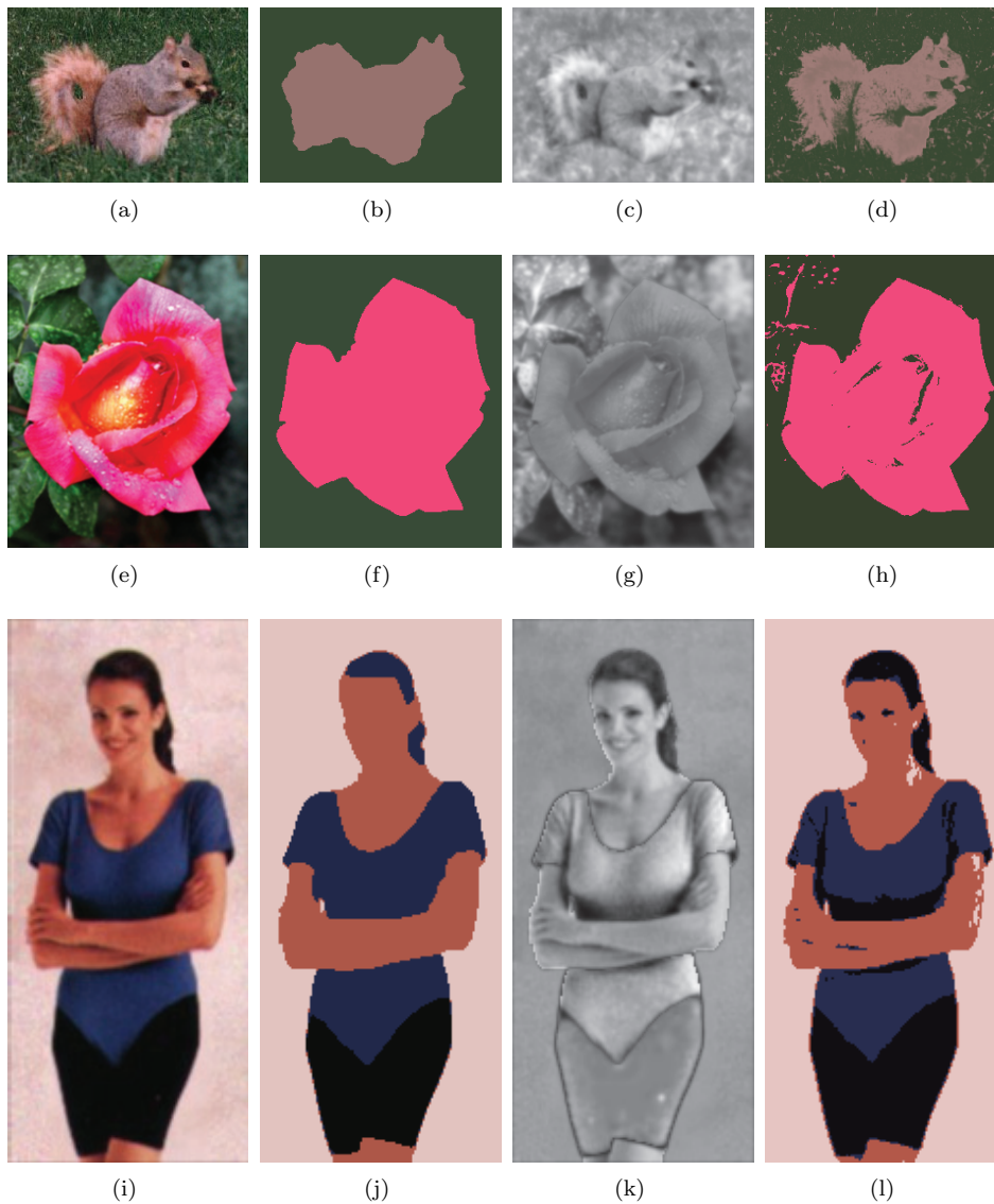
FIG. 5.6. The first column: test images; the second column: the segmentation by the proposed algorithm; the third column: the functions b in the proposed algorithm; the fourth column: the segmentation by the FCM algorithm. Parameters for squirrel image: \lambda = 0.0005, w = 0.001, \mu = 100 ; rose image: \lambda = 0.0005, w = 1, \mu = 10 ; woman image: \lambda = 0.01, w = 0.1, \mu = 10 .
