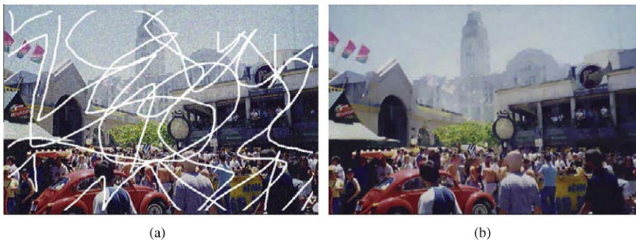
Fig. 6. Color image denoising and inpainting by the proposed algorithm. (a) Test image with mask which is contaminated by Gaussian noise with zero mean and standard deviation 20, size 591 \times 394 ; (b) denoised and inpainted image by our algorithm.
