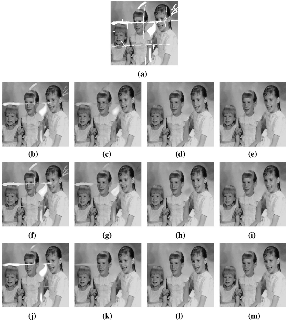
Fig. 1. Comparison of gray image inpainting algorithms. (a) The test image with inpainting mask (in white), size 256 \times 256 ; results of the proposed algorithm I: (b)–(d) intermediate inpainting results at iterations 20, 40 and 120; (e) final inpainted image at iteration 200, computational time = 3.7 s; results of the split Bregman algorithm: (f)–(h) intermediate inpainting results at iterations 20, 40 and 120; (i) final inpainted image at iteration 200, computational time = 6.5 s; results of the implicit TV inpainting algorithm in [13]: (j)–(l) intermediate inpainting results at iteration 100, 1000 and 3000; (m) final inpainted image at iteration 5000, computational time = 87.4 s.
