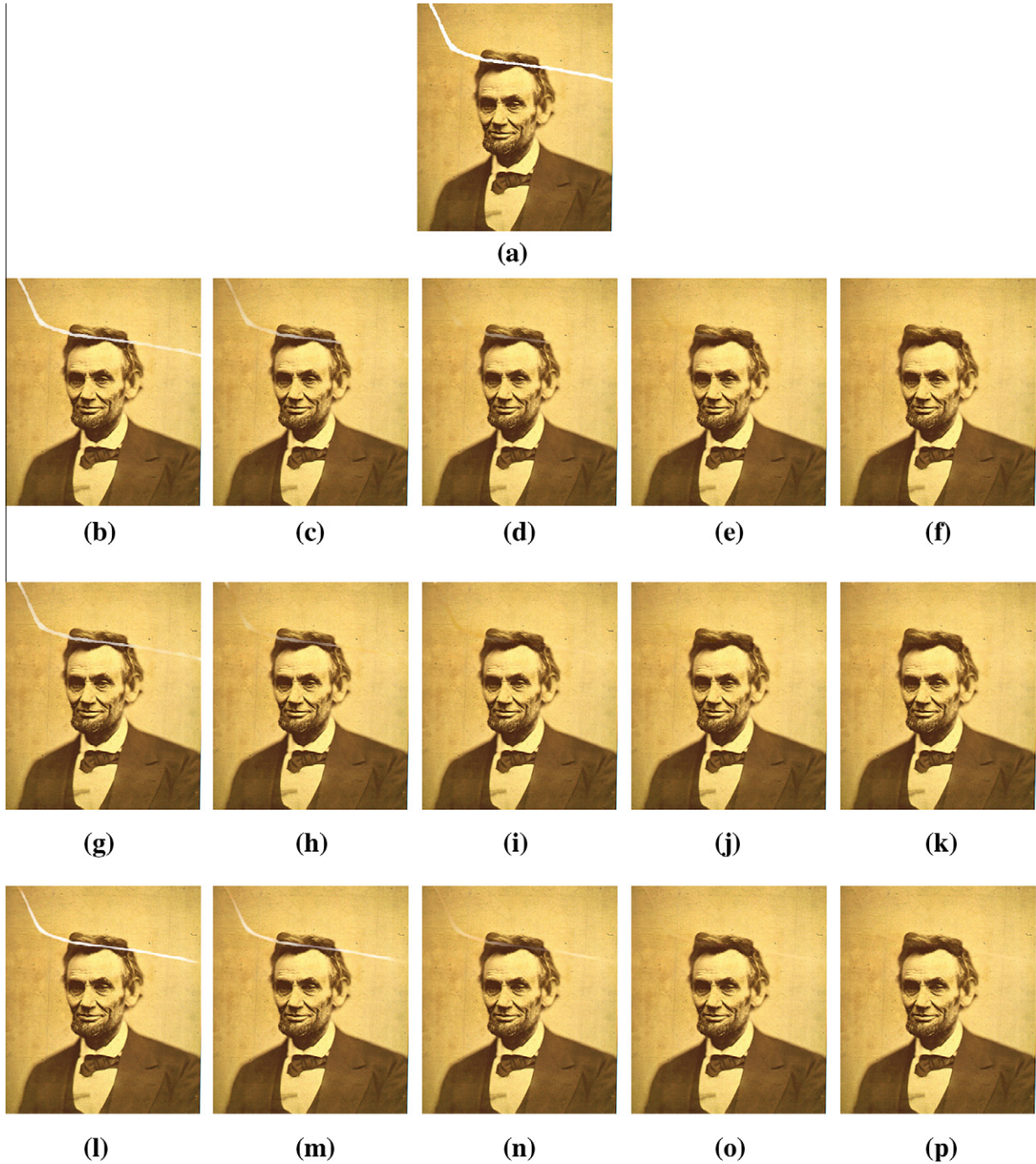
Fig. 4. Comparison of color image inpainting with algorithms. (a) The test image with mask, size 371 \times 432 ; results of algorithm II: (b)–(e) intermediate inpainting results at iterations 20, 40, 60 and 100; (f) final inpainted image at iteration 100, computational time = 14.7 s; results of the SB algorithm: (g)–(j) intermediate inpainting results at iterations 20, 40, 60 and 100; (k) final inpainted image at iteration 100, computational time = 20.9 s; results of implicit algorithm as in [13] for model (3): (l)–(o) intermediate inpainting results at iteration 100, 200, 400 and 1000; (p) final inpainted image at iteration 1500, computational time = 141.3 s.
