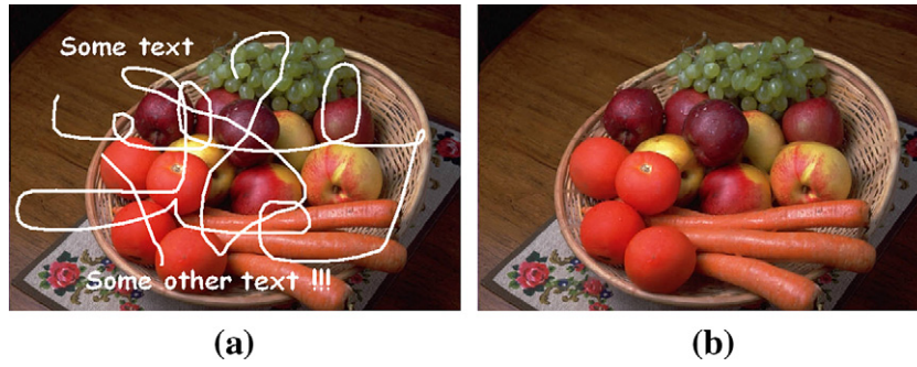
Fig. 7. Scratch removal by algorithm II. (a) Test image with mask, size 600 \times 406 ; (b) inpainted image.
