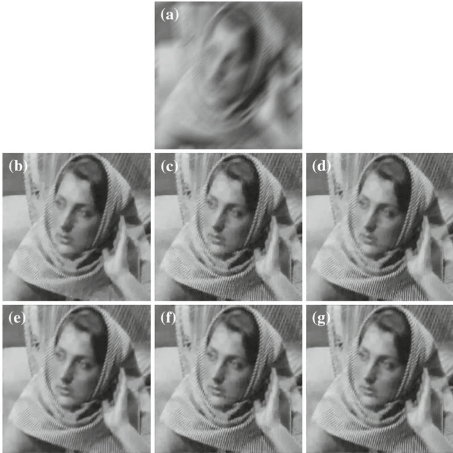
Fig. 6 Image deblurring. a Image corrupted by motion blur and Gaussian white noise of standard deviation 1; b Result of ROF, PSNR = 24.77 dB, iteration = 189, T = 4.6 s; c Result of TV+Local1, PSNR = 26.17 dB, iteration = 470, T = 37.1 s; d Result of TV+Local2, PSNR = 26.61 dB, iteration = 512, T = 139.5 s; e Result of FrameSB, PSNR = 26.23 dB, iteration = 126, T = 46.6 s; f Result of Algorithm 1'', PSNR = 26.94 dB, iteration = 726, T = 106.8 s; g Result of Algorithm 2, PSNR = 27.08 dB, iteration = 503, T = 183.4 s;
