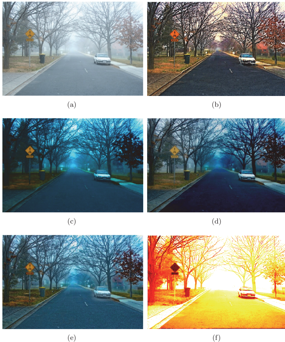
Figure 6. Comparison with other methods: (a) The original input hazy image ( 600 \times 400 ), (b) Tan's result, (c) Fattal's result, (d) He et al.'s result, (e) the proposed result, (f) the depth map using the proposed method.
