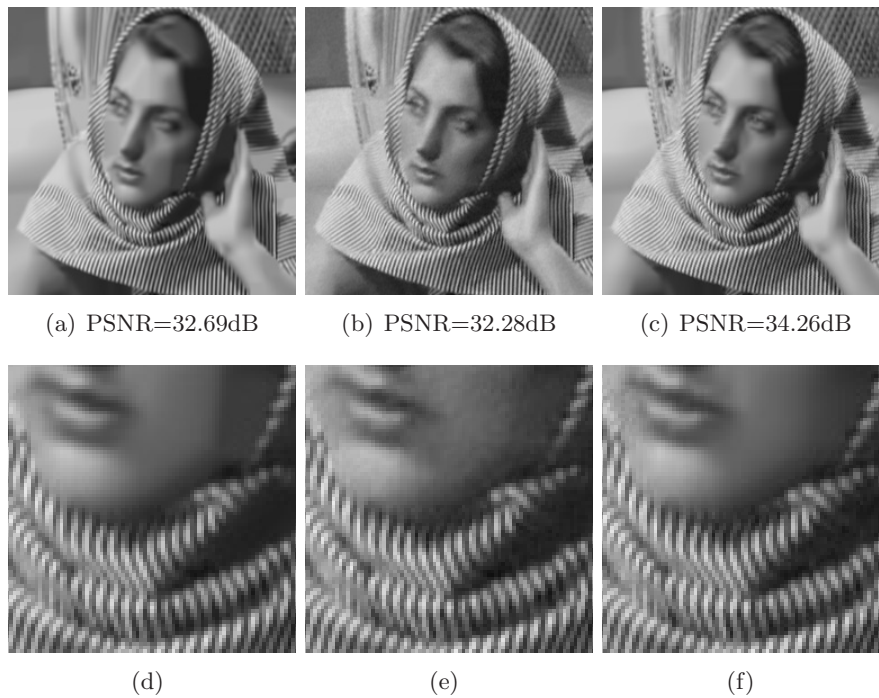
Figure 9. Fourier domain inpainting for Barbara with mask in Figure 2(b), sparsity = 30.72%, iteration = 3000. (a) ICTDI-BM3D; (b) ADMM-BM3D; (c) IDTDI-BM3D; (d)–(f) the zoomed regions of (a)–(c), respectively.
