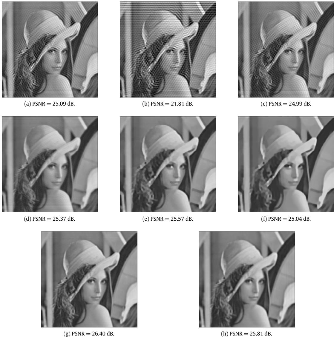
Fig. 3. Test on the blurred Lena image Fig. 1(b). (a) The result of IWF, iterations = 300, computational time = 170 s; (b) the result of IWF-Phase, iterations = 300, computational time = 228 s; (c) the result of IWF-ESTV, iterations = 300, computational time = 335 s; (d) the result of IWF-Phase&ESTV, iterations = 300, computational time = 375 s; (e) the result of method in [17], computational time = 97 s; (f) the result of method in [20], computational time = 161 s; (g) the result of the proposed IWF-H 1 , iterations = 245, computational time = 146 s; (h) the result of the proposed IWF-TV, iterations = 112, computational time = 172 s.
